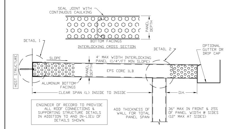
3" EPS ROOF PANEL/ SPAN DESCRIPTION
